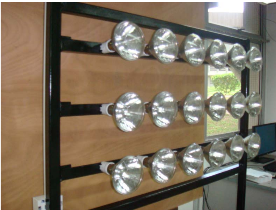
Figure 4.4b An array of light bulbs to simulate solar radiation
