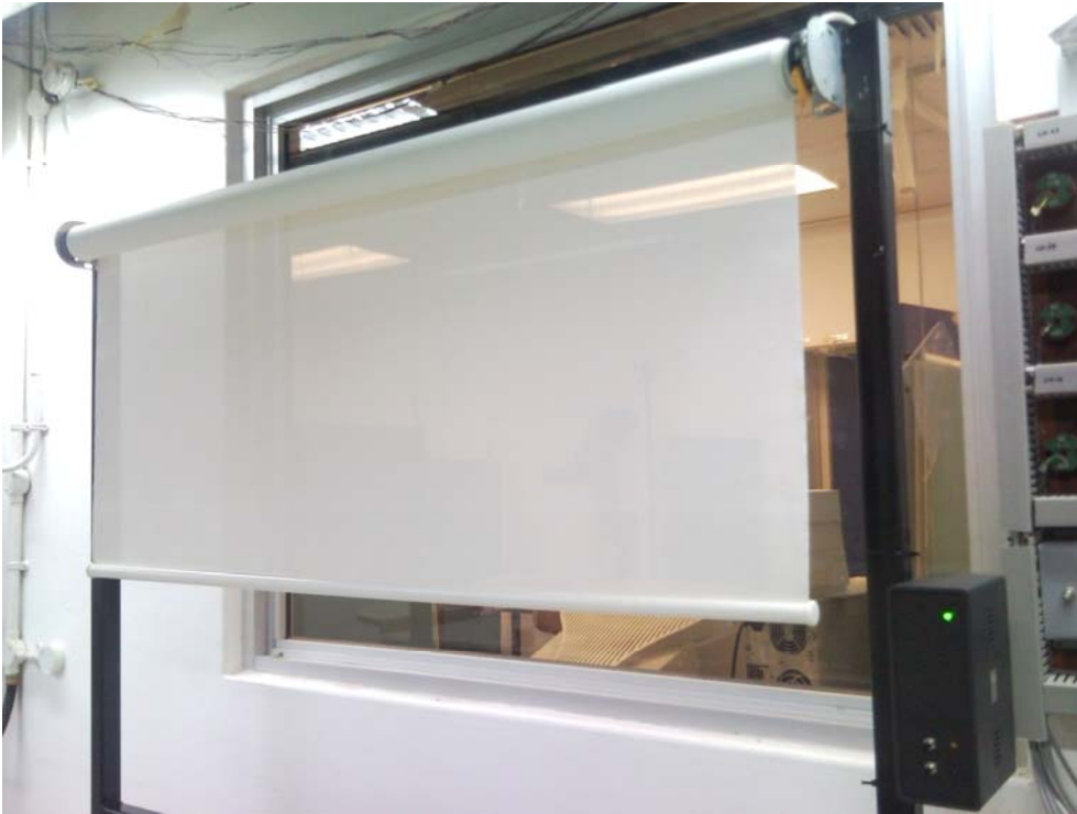
Figure 4.4a Laboratory prototype of a motorized window blind
