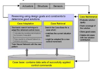
TSACS is the platform used to test the feasibility of optimisiation techniques and artificial intelligence for structural control.
